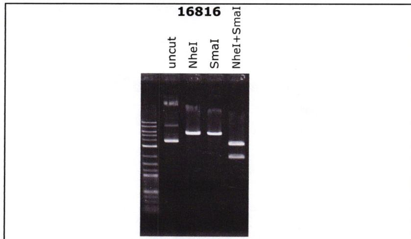
Electrophoresis : 100 nanogram DNA per lane ; 1% agarose gel , 1 x TAE Buffer
